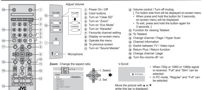
Hyper Scan: Press and hold . PR changes without changing the picture screen. Once you release the button, the picture of the selected PR will appear
